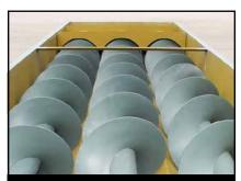
Screw Conveyor selection includes horizontal u-trough, tube screw and power pit feeder conveyors. Capacities range up to 6,600 bushels (168 metric tons) per hour.
