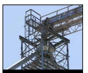
Distributor Turnheads are supported by two bearings instead of the standard single bearing. Cushion boxes and retarders are included to minimize grain damage at change of direction points.
