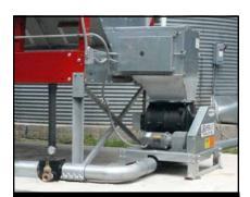
SUPER-AIR® Pneumatic System uses positive pressure to help move grain to multiple bins with just one power source. Choice of 4-, 5- or 6-inch (102-, 127- or 152-mm) diameter systems and capacities ranging up to 2,250 bushels (57.2 metric tons) per hour.
