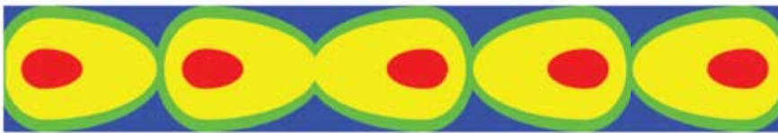
Heat pattern from typical tube-style heating system Note large cool blue areas and very hot red areas
